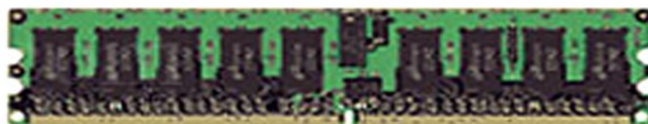
240 pin DDR-2 DIMM
