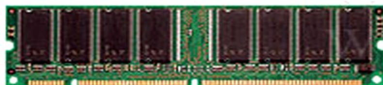
168 pin SDRAM DIMM
