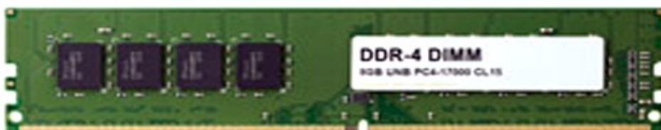
288 pin DDR-4 DIMM
